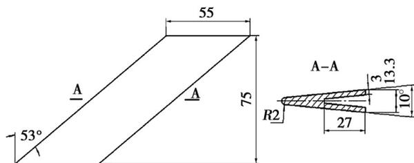
Fig. 2 Sketch of wing leading model
