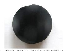
图 5 氧乙炔烧蚀 30 s 后的泡沫碳表面宏观形貌 Fig. 5 Surface macrograph of carbon foam after ablated for 30 s
