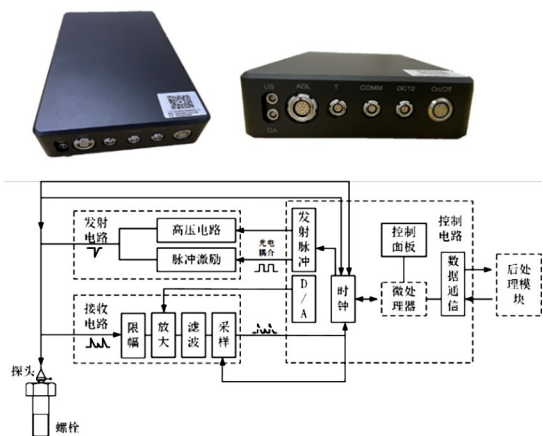
图4 螺栓预紧力测量设备及其结构示意图 Fig. 4 Schematic diagram of bolt preload measuring equipment and its structure
